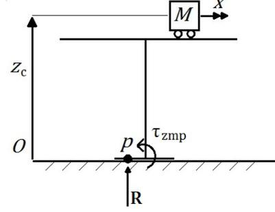
Fig. 2. Cart-table schematic
