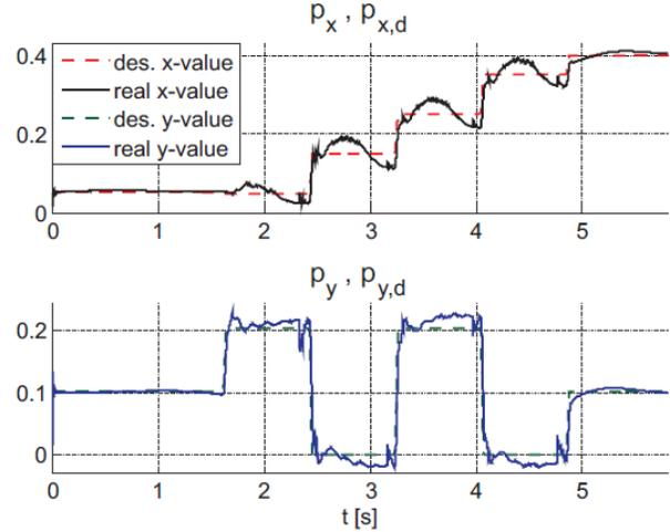
Fig. 9. preview ZMP controller in normal operation
