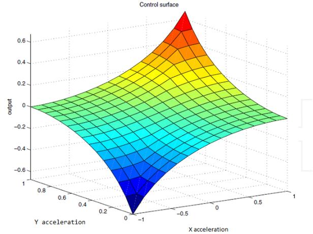
Fig. 8. fuzzy surface with  $x, y$  acceleration inputs
