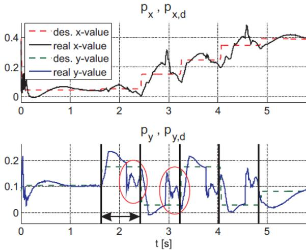
Fig. 11. preview ZMP controller with disturbance in 1.5 s
