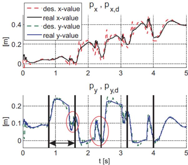
Fig. 12. fuzzy ZMP controller with disturbance in 1.5 s
