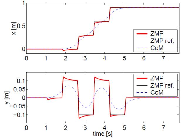
Fig. 6. ZMP and COM without disturbances (simulation).
