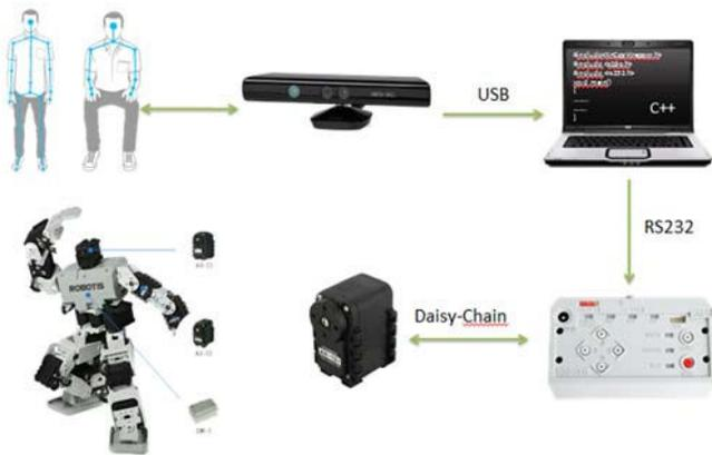
Figura 7. Sistema total Kinetic-Bioloid.
