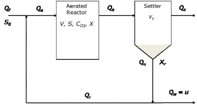
Figure 1 Activated sludge system.
