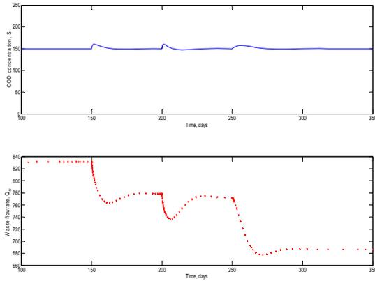
Figure 2 Control performance for regulation of COD and set-point change.
