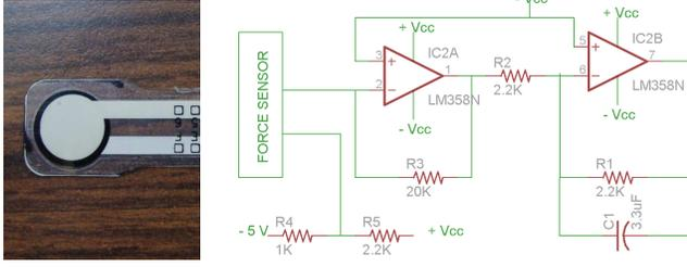
Figure 3. Flexiforce<sup>®</sup> Force Sensor (right), Conditioning Circuit (left)
