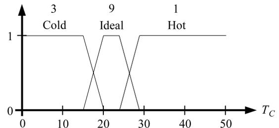
Figure 2. Membership functions of Temperature
