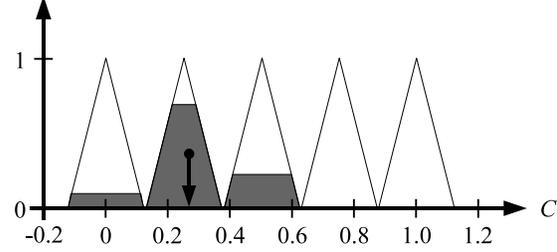
Figure 4. Aggregation of shot rules and defuzzification method
