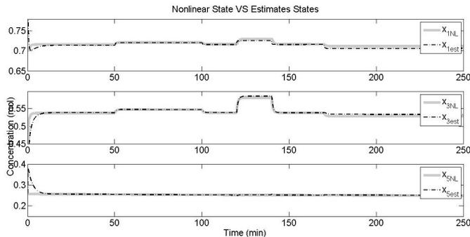
Figure 4. States of nonlinear system and estimated states.
