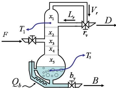
Figure 1. Scheme of a distillation column of five trays.
