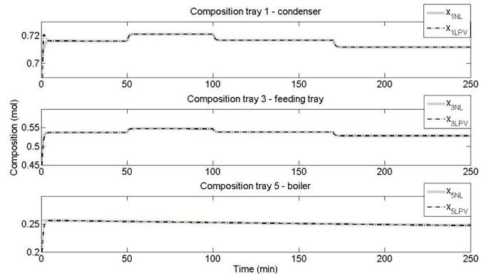
Figure 3. States of nonlinear system vs LPV singular model.
