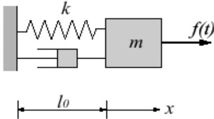
Fig. 1. Linear vibration of the ODF system
