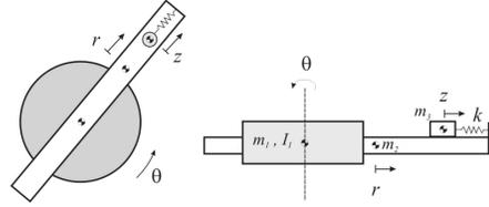
Fig. 3. Robot with oscillatory end-effector
