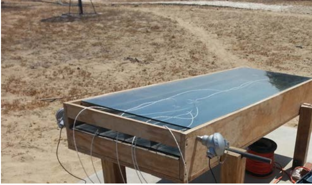
Fig. 2. Solar Collector with RTD Sensors
