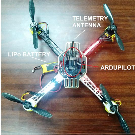
Fig. 2. The Quadrotor Storm Drone 4 and an Ardupilot onboard.
