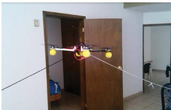
Fig. 9. Quadrotor hovering autonomously in a constrained indoor experiment.
