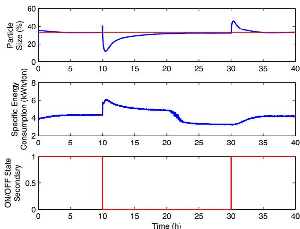
Fig. 8. Secondary line state change HMPC
