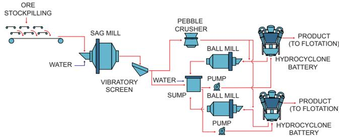
Fig. 1. Schematic of the simulated plant
