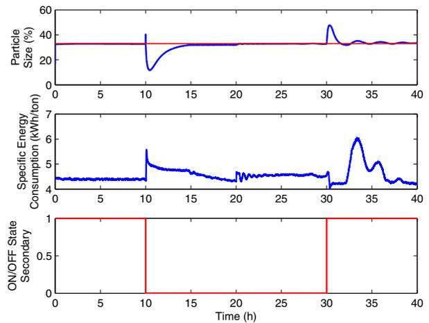
Fig. 6. Secondary line state change CMPC
