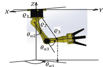
Fig. 1. Manipulator arm with three degrees of freedom.
