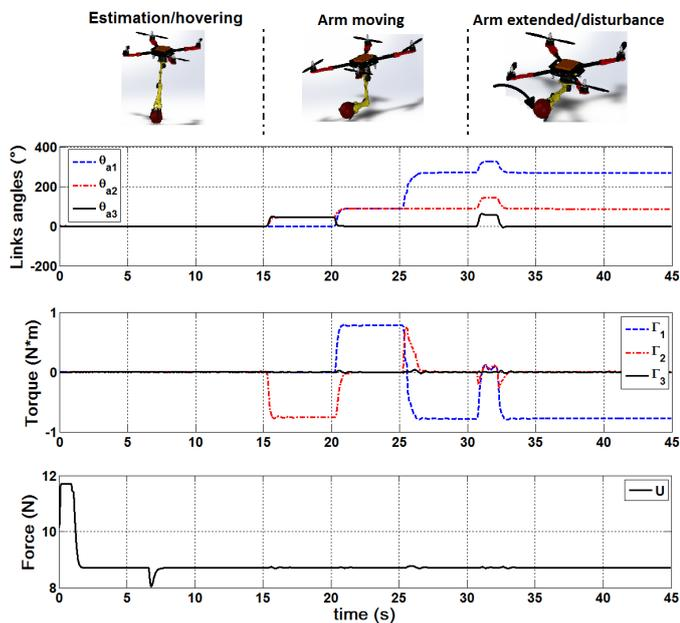
Fig. 4. Angular positions of the links of the manipulator, control torques and thrust signals during the simulation.
