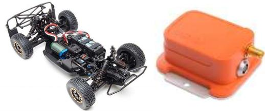
Fig. 2. Car-like WMR and Xsens sensor.
