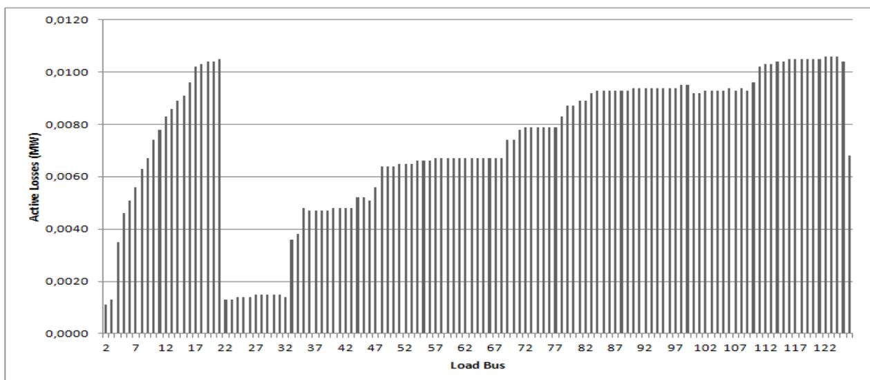
Figure. 5. Variation of active power losses for the system of 126 bus with an increase of 100kW at load buses.
