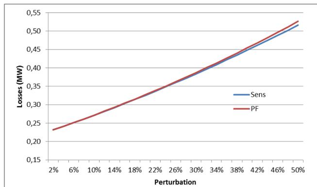
Figure 2. Comparison of active power losses of 34 bus system.
