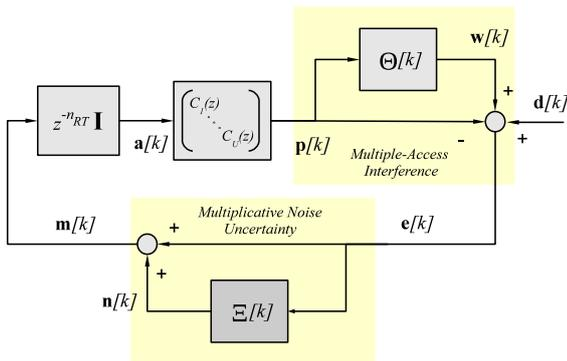
Fig. 2. Overall Closed-Loop Structure for Power Allocation.
