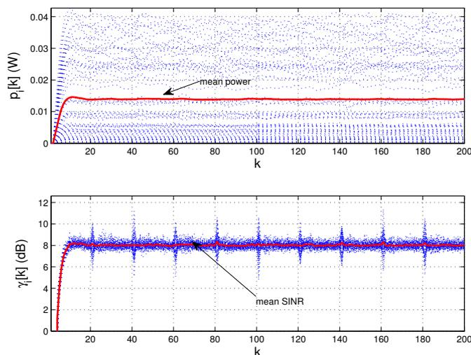
Fig. 4. Performance of Power Allocation Scheme for 4 BSs.
