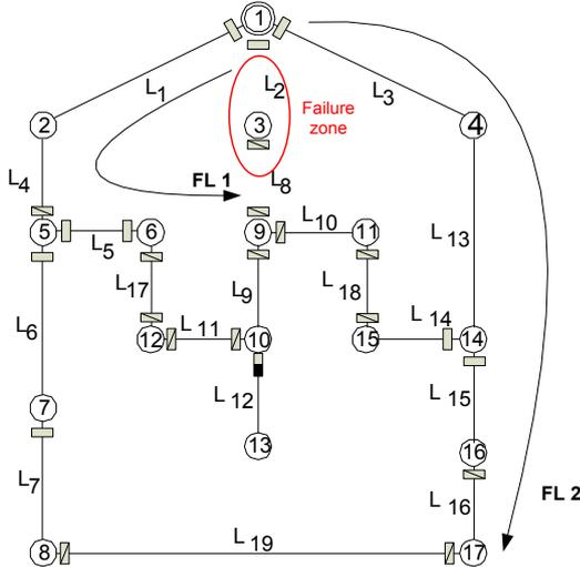
Fig. 2 Civanlar system with fault on line 2.
