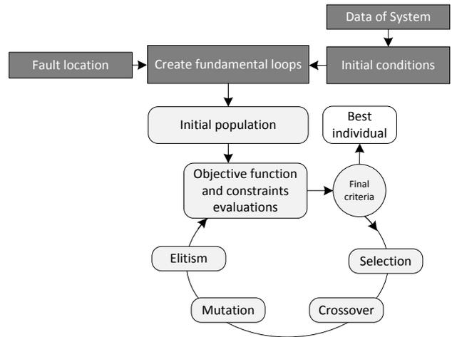
Fig. 4. Block Diagram of the proposed GA
