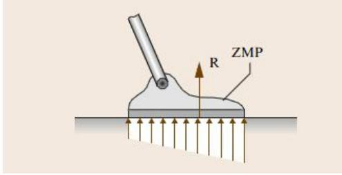
Fig. 1. Original definition of the zero-moment point (ZMP), (Siciliano et al., (2008)).
