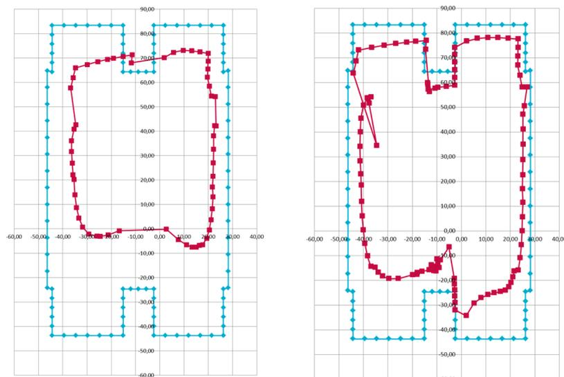
Fig. 6. ZMP safety zone in red obtained with a 10% error on the left and 5% error on the right.
