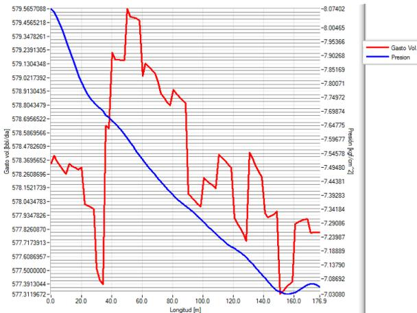
Fig. 4. Profiles of flow-rate (left in [bpd]) and pressure (right in  $[\frac{kgf}{cm^2}]$ ) along the pipeline (length in [m]) without any leak.
