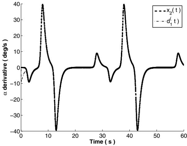
Fig. 3. Estimation of velocity for the angle  $\alpha(t)$  based on the STA applied as STA. The estimated velocity is compared with the measured velocity obtained from the model exported to Matlab.
