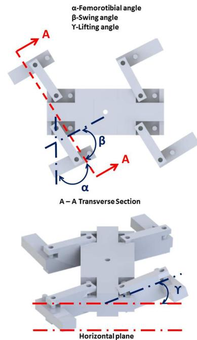
Fig. 2. Simplified model used to represent the angles of one GIR single leg evaluated in the numerical simulations of this study.
