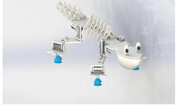
Fig. 1. GIR model used to construct the numerical simulations of this study. This model is built in SolidWorks and then exported to Matlab. All the simulations are executed in the SimMechanics Toolbox®
