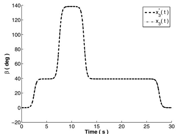
Fig. 6. Tracking trajectory of second link in the left rear leg of GIR. The solid line represents the reference trajectory and the dashed line corresponds to the trajectory of the actual joint angle.
