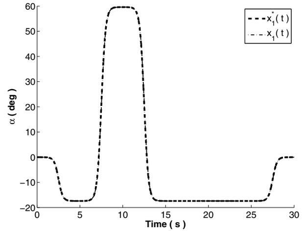
Fig. 5. Tracking trajectory of first link in the left rear leg of GIR. The solid line represents the reference trajectory and the dashed line corresponds to the trajectory of the actual joint angle.
