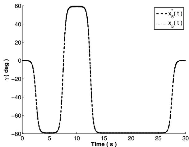
Fig. 7. Tracking trajectory of second link in the left rear leg of GIR. The solid line represents the reference trajectory and the dashed line corresponds to the trajectory of the actual joint angle.
