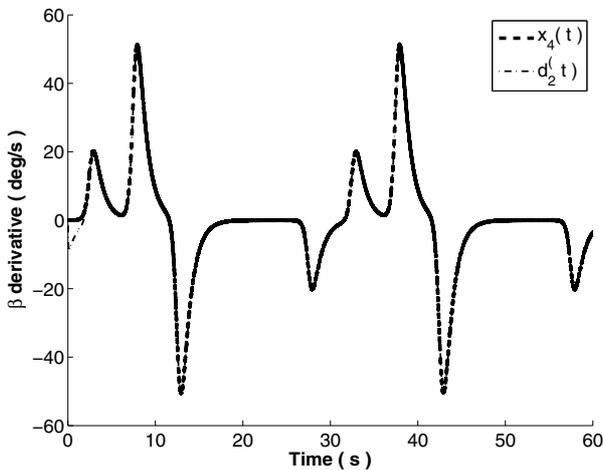
Fig. 4. Estimation of velocity for the angle  $\beta(t)$  based on the STA applied as STA. The estimated velocity is compared with the measured velocity obtained from the model exported to Matlab.
