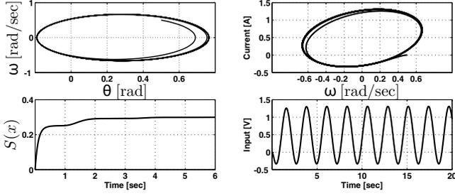
Fig. 2. Closed-loop response of the DC-motor actuated pendulum system.
