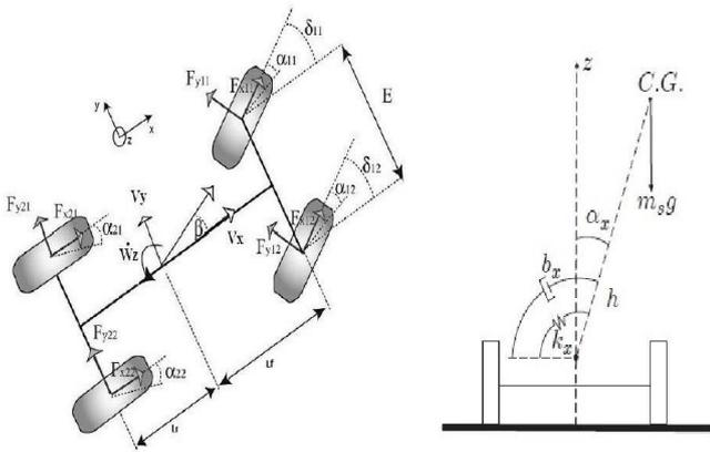
Fig. 1. Four Wheels Vehicle Model with Roll Dynamic
