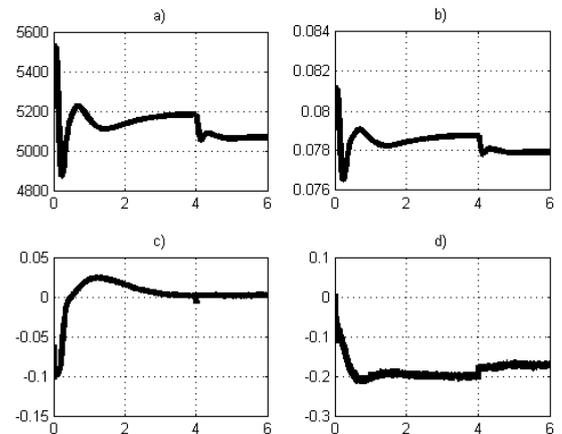
Fig. 4. a) Vertical tyre force  $F_{z,11}$  [N vs s]; b) contact patch length  $a$  [m vs s]; c) measured longitudinal acceleration  $a_x$  [g's vs s]; d) measured lateral acceleration  $a_y$  [g's vs s].
