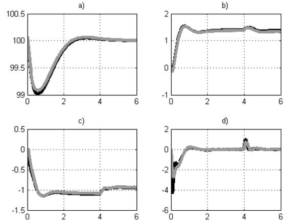
Fig. 3. a) Real longitudinal velocity  $v_x$  (black) and estimation  $\hat{v}_x$  (gray) [km/h vs s]; b) real lateral velocity  $v_y$  (black) and estimation  $\hat{v}_y$  (gray) [km/h vs s]; c) real roll position  $\alpha_x$  (black) and estimation  $\hat{\alpha}_x$  (gray) [deg vs s]; d) real roll rate  $w_x$  (black) and estimation  $\hat{w}_x$  (gray) [deg/s vs s].
