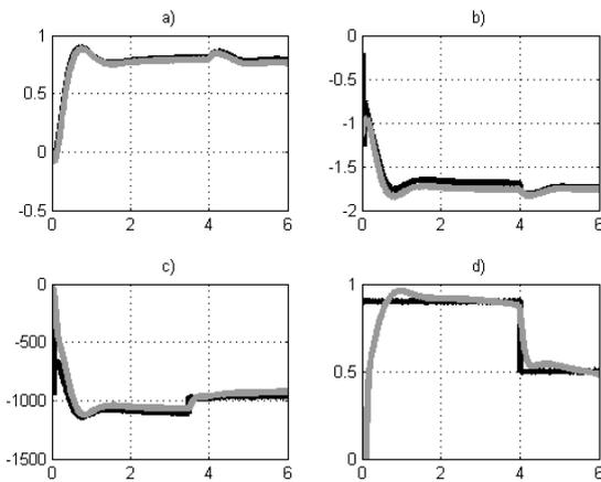
Fig. 5. a) Real sideslip angle  $\beta$  (black) and estimation  $\hat{\beta}$  (gray) [deg vs s]; b) real tyre slip angle  $\alpha_{11}$  (black) and estimation  $\hat{\alpha}_{11}$  (gray) [deg vs s]; c) real tyre lateral force  $F_{y,11}$  (black) and estimation  $\hat{F}_{y,11}$  (gray) [N vs s]; d) real tyre-road friction coefficient  $\mu_y$  (black) and estimation  $\hat{\mu}_y$  (gray) [adimensional vs s].
