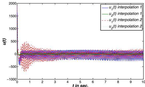
Fig. 10. Control law  $u(t)$  for the two-parameter feedback configuration of  $K(\theta(t))$  applied to  $P(\theta(t))$
