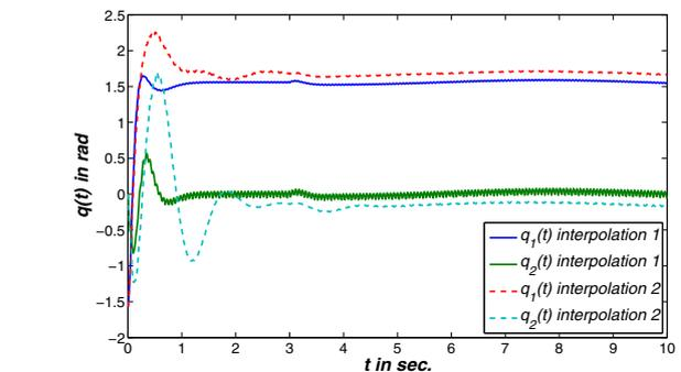
Fig. 9. Positions  $q(t)$  for the two-parameter feedback configuration of  $K(\theta(t))$  applied to the non-linear model
