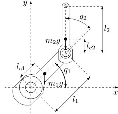
Fig. 3. Two DOF planar rotational robot.
