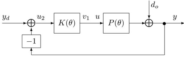
Fig. 1. Feedback system with one-parameter controller.
