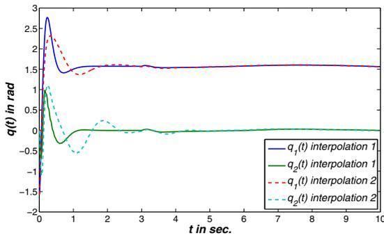
Fig. 5. Positions  $q(t)$  for the one-parameter feedback configuration of  $K(\theta(t))$  applied to the non-linear model
