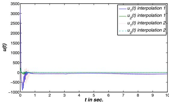
Fig. 6. Control law  $u(t)$  for the one-parameter feedback configuration of  $K(\theta(t))$  applied to  $P(\theta(t))$
