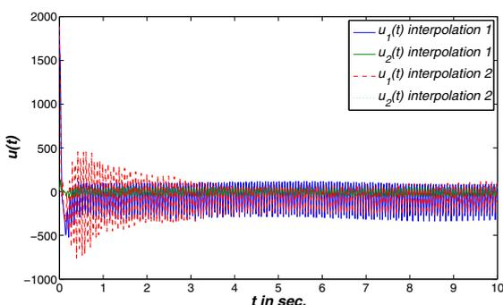
Fig. 11. Control law  $u(t)$  for the two-parameter feedback configuration of  $K(\theta(t))$  applied to the non-linear model
