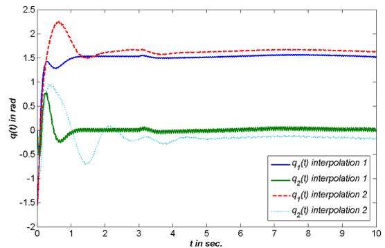
Fig. 8. Positions  $q(t)$  for the two-parameter feedback configuration of  $K(\theta(t))$  applied to  $P(\theta(t))$
