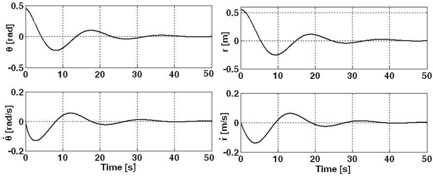
Figure 3. Closed-loop response of the **BBS** to the initial conditions: **a)**  $x_0 = (0.55\text{m}; 0; 0.45\text{rad}; 0)$
