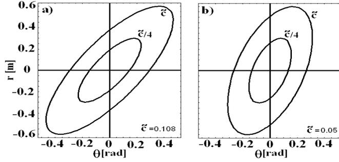
Figure 2. Level curves of the function  $\Phi(q)$  around the origin, for two sets of values;  $\bar{n}\bar{k} = 1$ ,  $\delta = 0.015$  and  $k_p = 2.5$  (left) and  $\bar{n}\bar{k} = 1$ ,  $\delta = 0.015$  and  $k_p = 1.3$  (right). With restrictions on  $|r| \leq 0.6[\text{m}]$  and  $|\theta| \leq 0.5[\text{rad}]$ .
