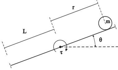
Figure 1. The ball and beam system.
