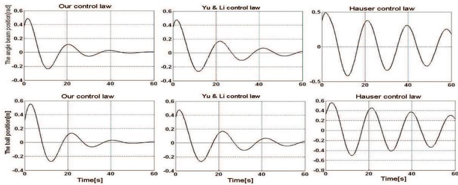
Figure 4. Closed-loop response of the **BBS** to the proposed **ANC** in comparison with **YNC** and **HNC**.
