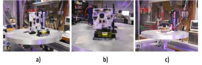
**Figure 9. IMU rotations to calibrate each rate gyro, a) for the x-axis, b) for the y-axis and c) for the z-axis**
