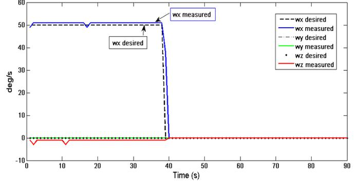
**Figure 11. Comparison between the simulated and measured angular velocity  $\omega_x$ .**
