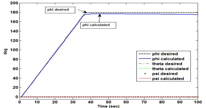
**Figure 12. Comparison between the simulated and the calculated  $\phi$  Euler angle**
