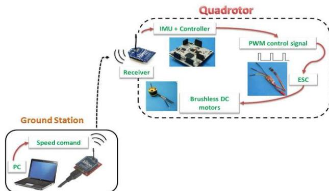
Figure 13. Block diagram for the open loop flying test
