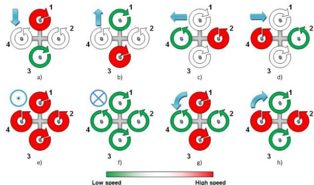
**Figure 1. Different Quadrotor maneuvers depending on the speed and direction of the blades rotation**
