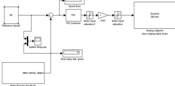
**Figure 8. Simulink® block diagram for the PID controller of the CRT**
