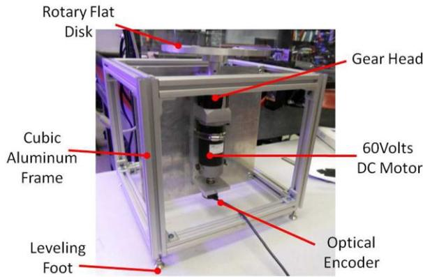
**Figure 7. IMU calibration platform**
