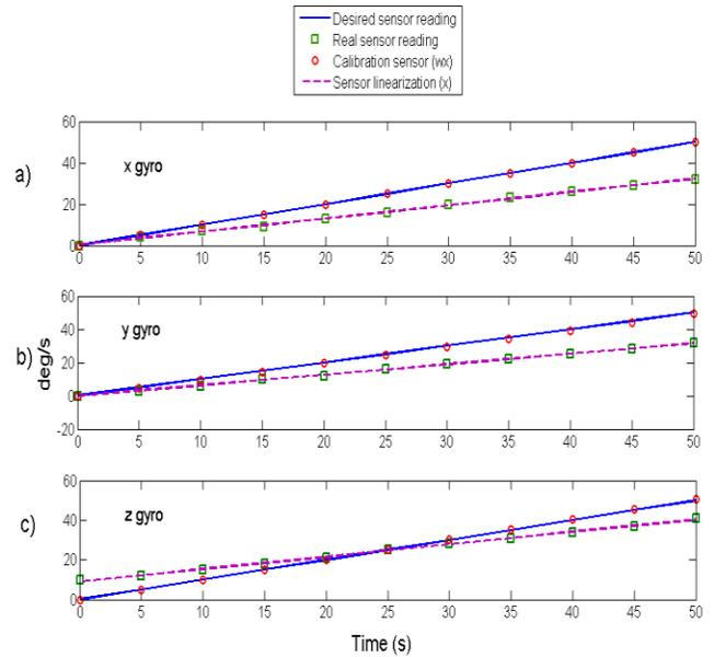
**Figure 10. Rate gyros performance during the calibration process**
