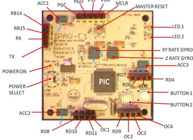
**Figure 6. Components of the IMU**
