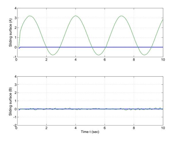
Fig. 2. Column (A) shows the system without compensation and in column (B) the compensated system
