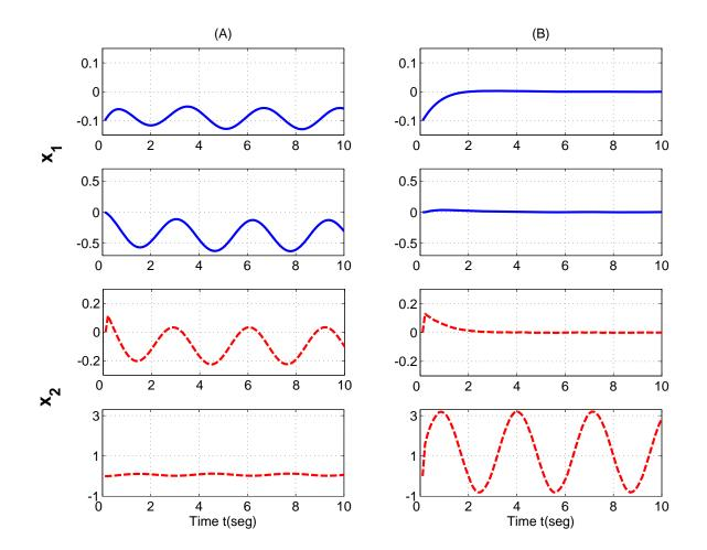
Fig. 1. Column (A) shows the canonical form system without compensation and in column (B) the compensated system. The underactuated states are plotted in solid-line, while the completely actuated states are plotted in (dashed-line)
