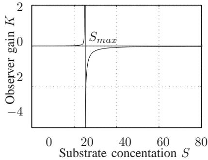
Figure 5. Qualitative behavior of the right hand side of assessment on  $K$  in dependence on the substrate concentration  $S$  for  $\epsilon \ll 1$ .
