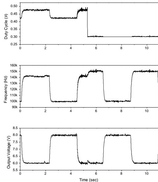
Figure 4. Time evolution of the converter under parallel control, at time  $t = 5.3\text{sec}$  the duty-cycle input saturates.
