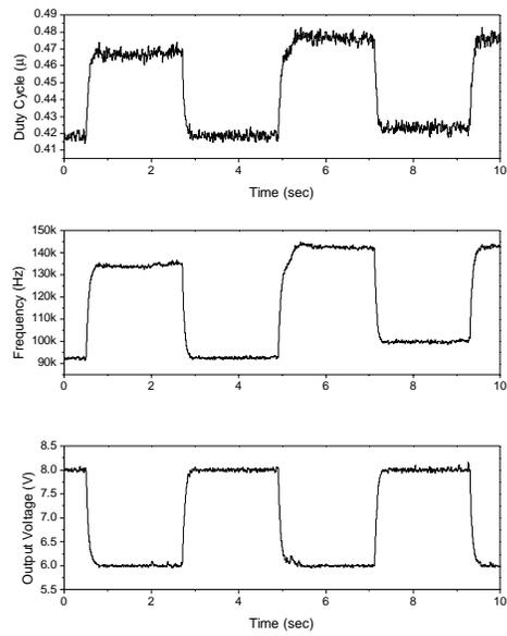
Figure 5. Time evolution of the converter under parallel control when a load disturbance occurs at  $t = 4$  sec .
