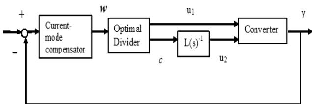
Figure 1. Schematic diagram of parallel control.
