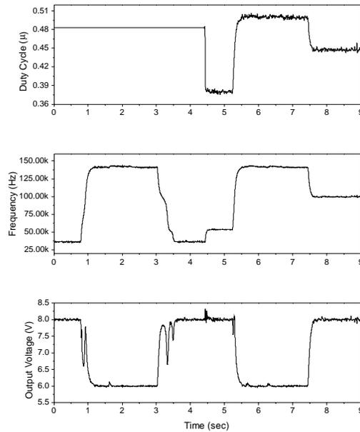
Figure 3. Time evolution of the converter under a) ( $t < 4.5\text{sec}$ ) single input control law b) ( $t \geq 4.5\text{sec}$ ) parallel control.
