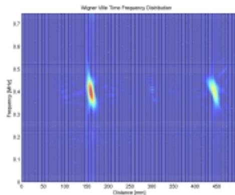
**Fig. 11. Echo-Pulse Signal Processed by using TFD with First Flaw**
