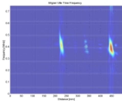
**Fig. 12. Echo-Pulse Signal Processed by using TFD with Second Flaw**
