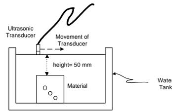
Fig. 3 Schematic Diagram of Setup Experiment
