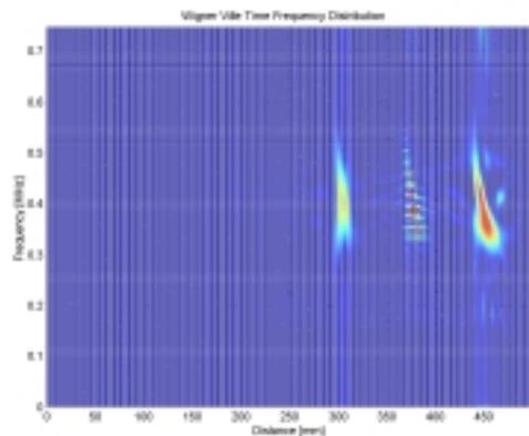
**Fig. 13. Echo-Pulse Signal Processed by using TFD with Third Flaw**
